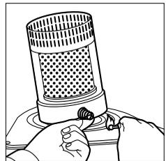
**NOTE:** An improperly seated heat chamber can cause high flame, smoke, and potential damage to the heater itself. Do not leave the heater until you have determined that the flame is burning normally, will be described in the following section.
